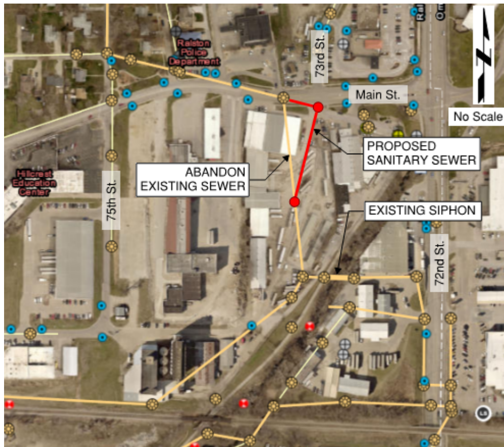
Figure 3-2: 73 rd Street Sanitary Sewer Relocation
