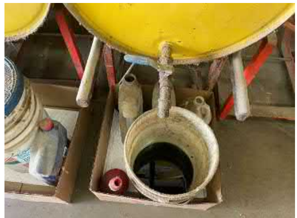
Photo #18 View of one of several drip pans located beneath the drums located in the maintenance shop.
