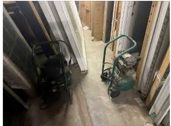
Photo #10 View of two of ten portable air compressors located in the AAA Building Components warehouse space
