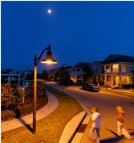
An example of a full cutoff fixture
